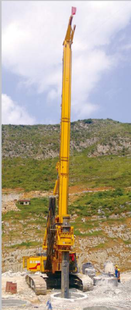
徐工XR460D旋挖钻机大战灰岩 XCMG XR460D was fighting against limestones
