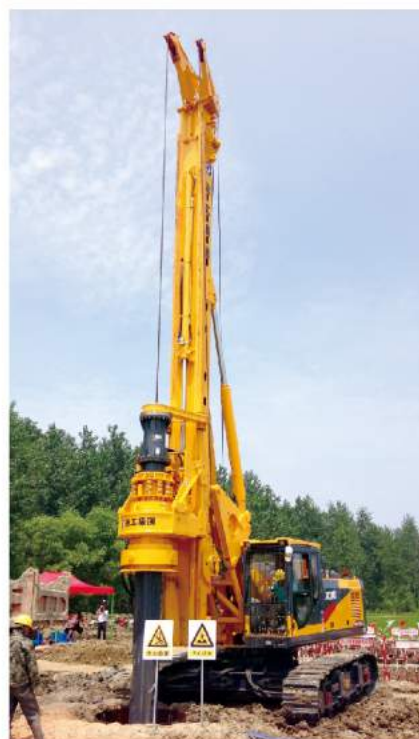
徐工旋挖钻机助力国家电网淮南-南京-上海工程线路工程 XCMG rotary drilling rigs are working in Huainan- Shanghai Railway Project
